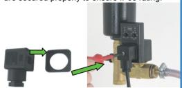
6. After double checking that the power supply corresponds with the voltage specified on the coil and falls within the range specified on the back of the timer, you can switch the power supply ON.
