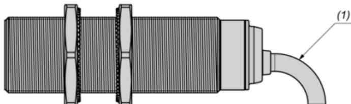
(1) Bending cable: 4 x external cable diameter
