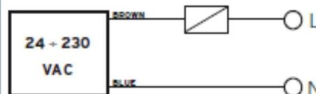
Warning: Short circuit in the output is not possible. Wrong supply cables connections can irreparably damage the detector. Therefore sensors whose output status is short-circuited will not be substituted under warranty.
