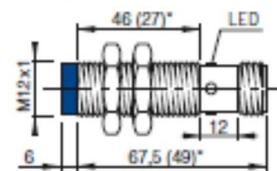
(\*) The dimensions into brackets refer to short housing models.
