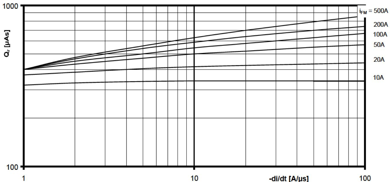
Sperrverzögerungsladung / Recovered charge  $Q_r = f(-di/dt)$  $T_{vj} = T_{vjmax}$ ,  $V_R \leq 0,5 V_{RRM}$ ,  $V_{RM} = 0,8 V_{RRM}$ Parameter: Durchlaßstrom / On-state current  $i_{FM}$
